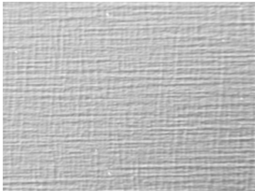
RTD surface on Ge/Si substrates, roughness \sim 7 nm
